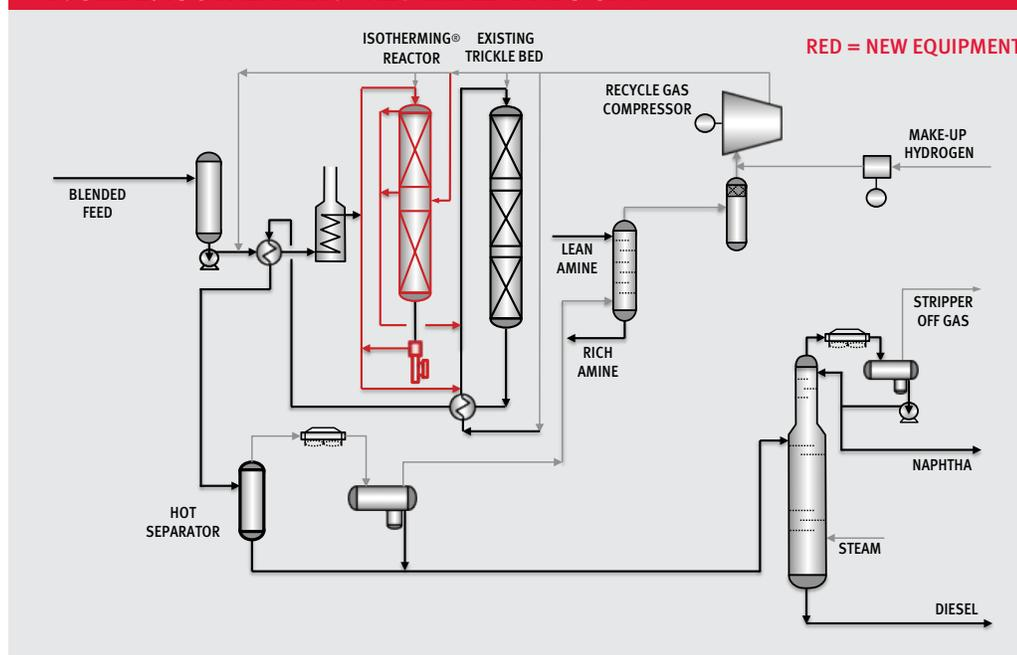
cycle oil (LCO) or coker gas oil (CGO), the low temperature rise across the IsoTherming® reactor system provides a particular advantage not only due to decreased uncontrolled cracking, but allows for effective treatment of hard to remove nitrogen compounds without sulfur recombination.
